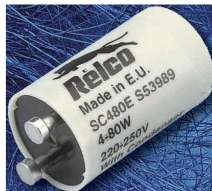
Modified in such a way, the excited gases in the bulb generate some 240 evaluable emission lines. Counting also those on all overlapped Echelle orders, this number increases even to approximately 370. Between the individual starters, the intensity of the hydrogen Balmer series can vary very strongly. Numerous additional lines, which are not listed here, are gen-
